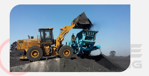
Mobile Jaw Crushers are used to crush so that we can reduce and liberate the clean coal from the shale or any gangue material.
